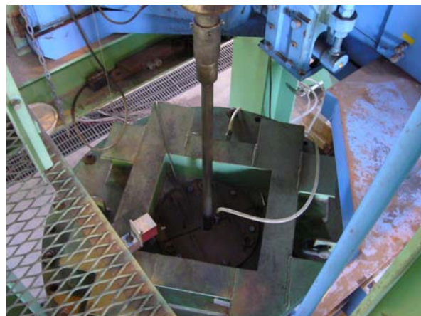
Photo 2.15 Cone penetration test
