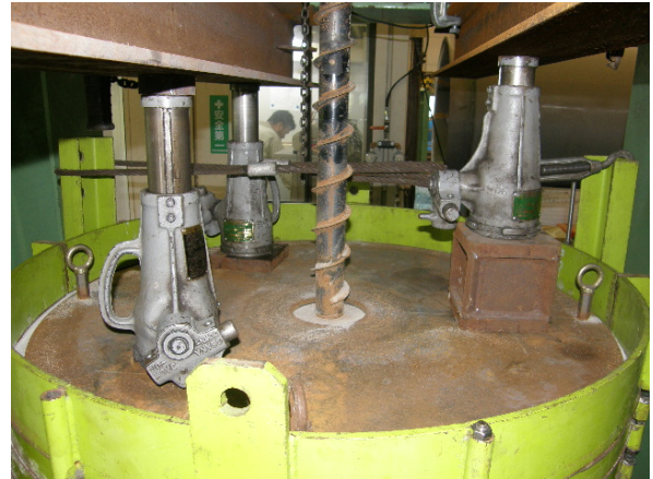
Photo 2.23 Loading overburden pressure
