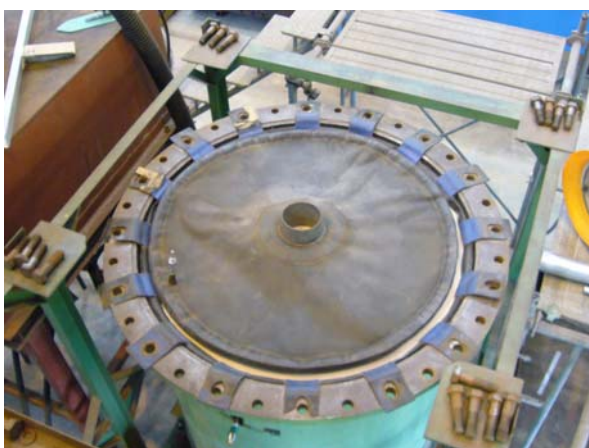
Photo 2.11 Installation of the air bag
