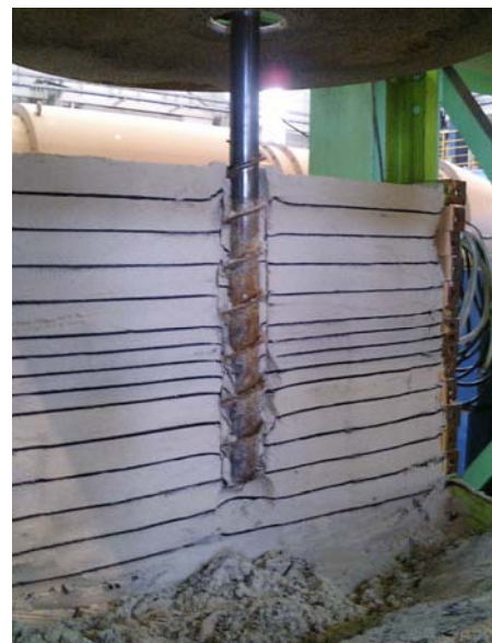
Photo 2.27 Loading on pile head
