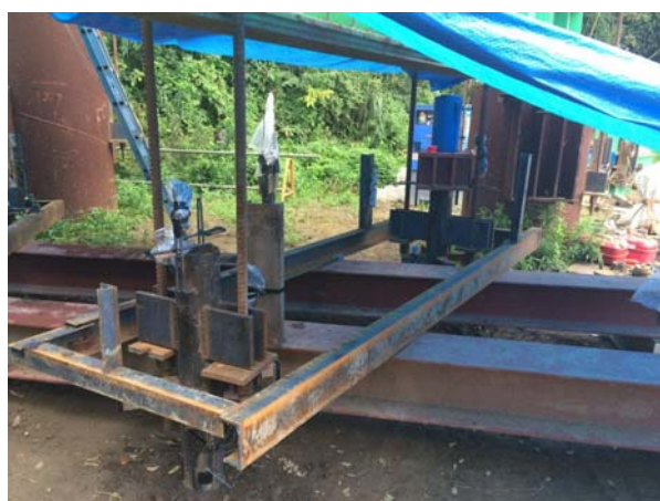
Photo 5.6 Monotonic tensile loading (B-MT)
