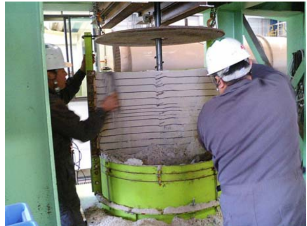
Photo 2.25 Cutting sand ground
