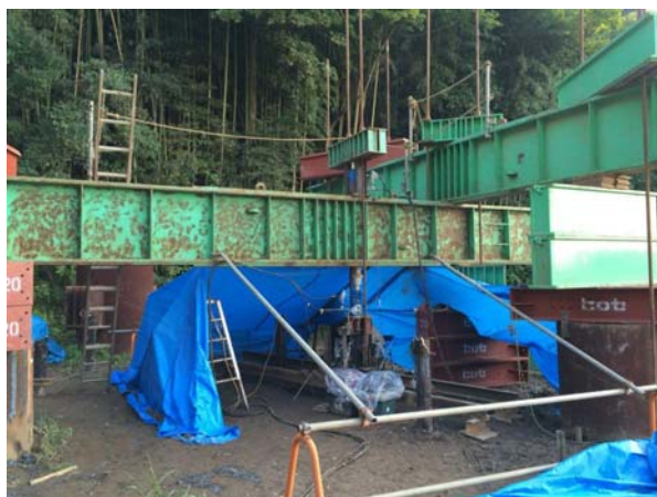
Photo 5.7 Cyclic reversal loading
