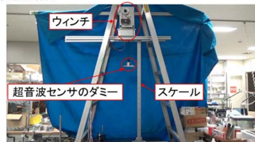
Fig. 9: Experiment of position control of a dummy sensor
