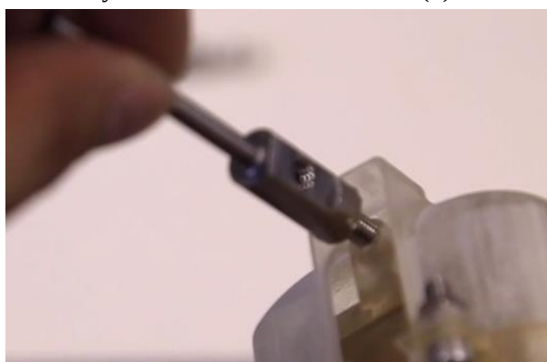
(c) screwing the nozzle into the drain separator
