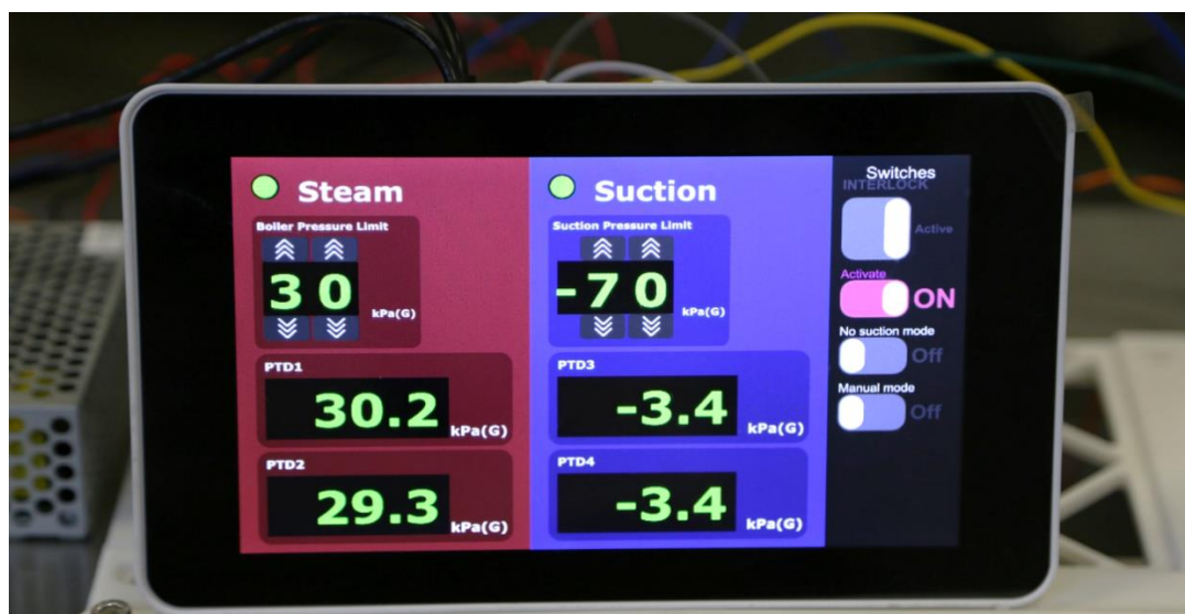
Fig. 3.20 Apparatus of the developed control panel with 7-inch touchscreen LCD
