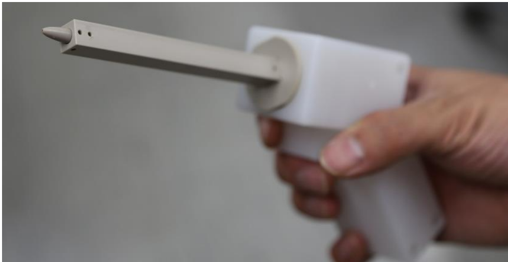
Fig. 2.13 Apparatus of fabricated steam jet nozzle unit of the research prototype
