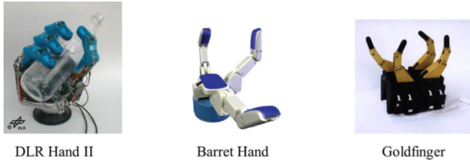
Figure 1-6: Robotic hand that has actuator installed at the joint (Image from [10, 11, 12])
