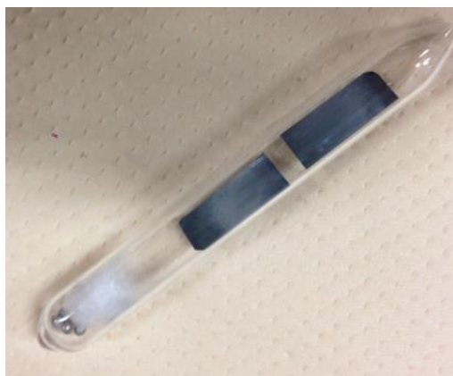
Figure A2.2 the vacuum sealed silica glass tube with pure Zn beads and Cu/Ti electrodes inside.
