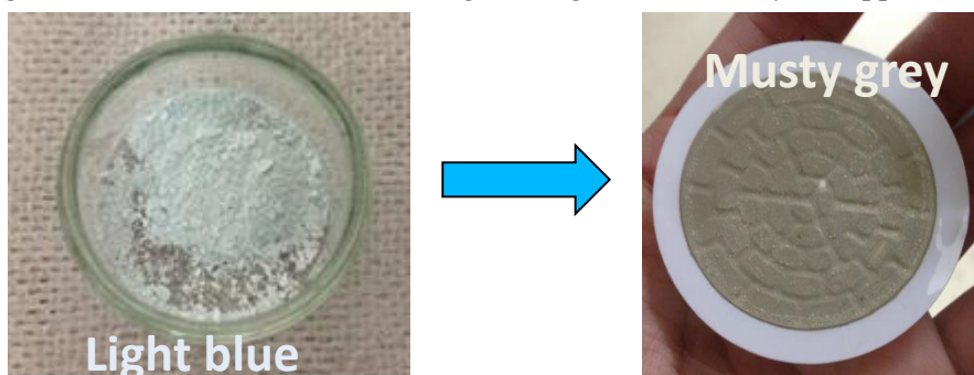
Figure 2.16 The color change of \text{Cu}_x\text{O} nanoclusters-grafted \text{Nb}_3\text{O}_8^- nanosheets before and after the UV irradiation.
