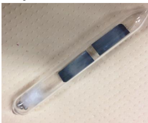
Figure 3.2 the picture of the sealed glass tube with Zn metal grains and annealed Cu-Zn film inside.
