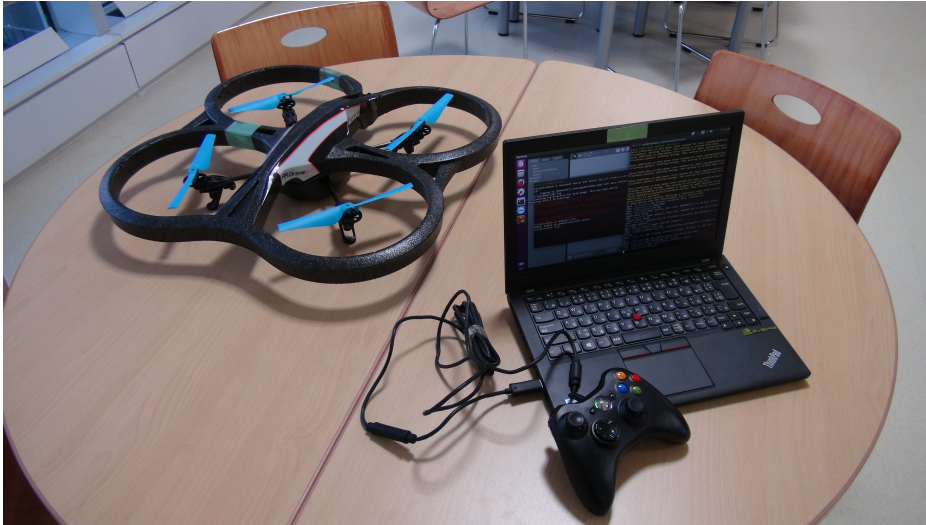
Fig. 3.5 Hardware equipment setup for training the SOIAM based controller, including a ground control laptop that exchanges sensing data and control command with AR.Drone through Wi-Fi ad-hoc network. An XBOX gaming controller generates commands from human demonstration for training.
