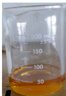
Figure 4-6 The harmonious state of CD cracked oil/biodiesel=1:50
