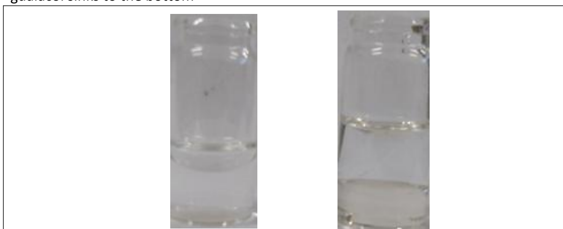
Figure 4-7 Mixing results of benzene(left) and guaiacol(right) with water
