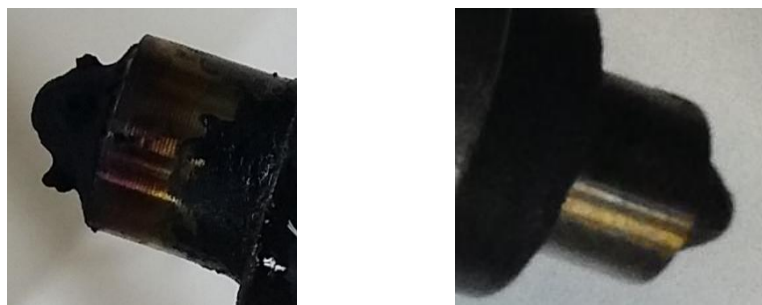
Figure 2-27 Nozzle tip : right (before the test) and left (after the test)
