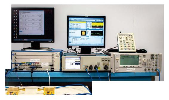
Figure 5.32: Setup for transmitter-to-receiver wireless communication error vector magnitude (EVM) measurements photo.
