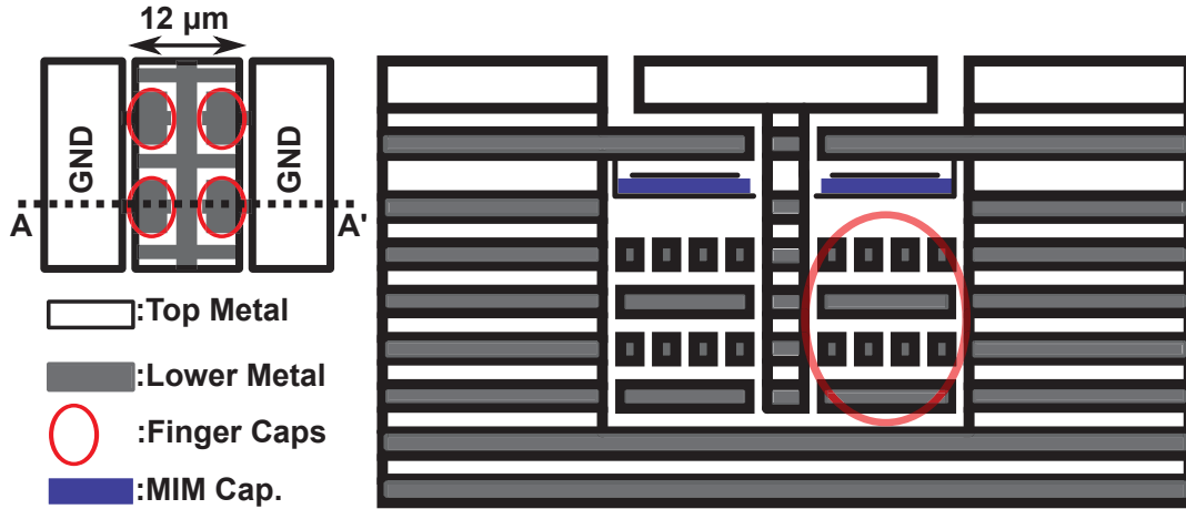
Figure 3.19: Illustration of metal layers and MIM capacitor layers for MIM transmission line.
