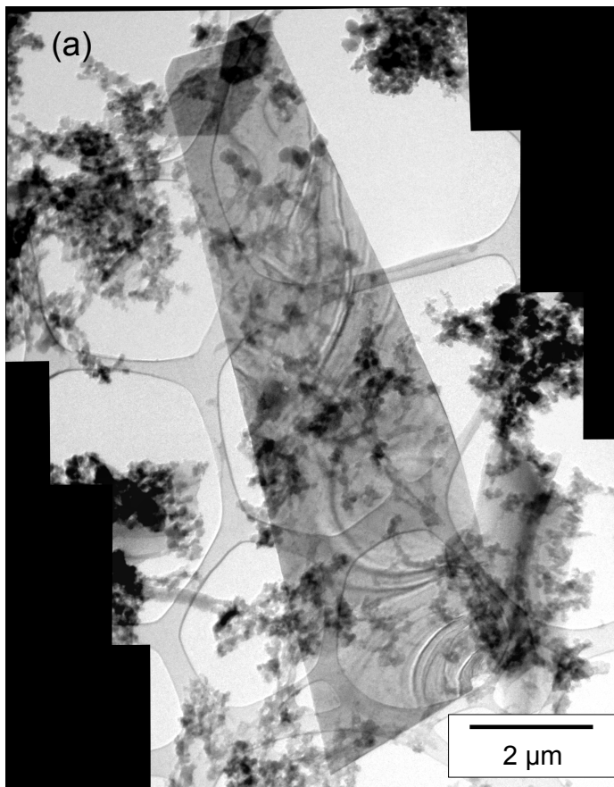
Fig. 6. 8 (a) TEM bright field image and (b) schematic illustration showing a transformed region and strain contrast in a plate-like precipitate extracted from the as-homogenized sample.
