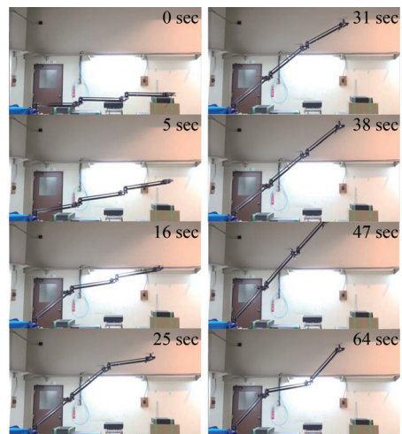
Fig.7 Pitch joint control experiment.
