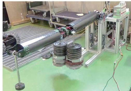
Fig. 18 Experiment with heavy load of 142.4kg applied to two units prototype model.
