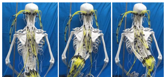
Fig. 5 Side bending of the back mechanism (left: natural state, middle: left side bending, right: right side bending).
