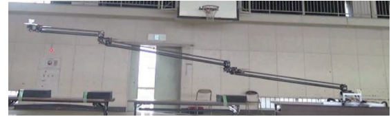
Fig. 18. Experiment with 5 meters model (lengths of the first and second proximal links are 2.0 m).
