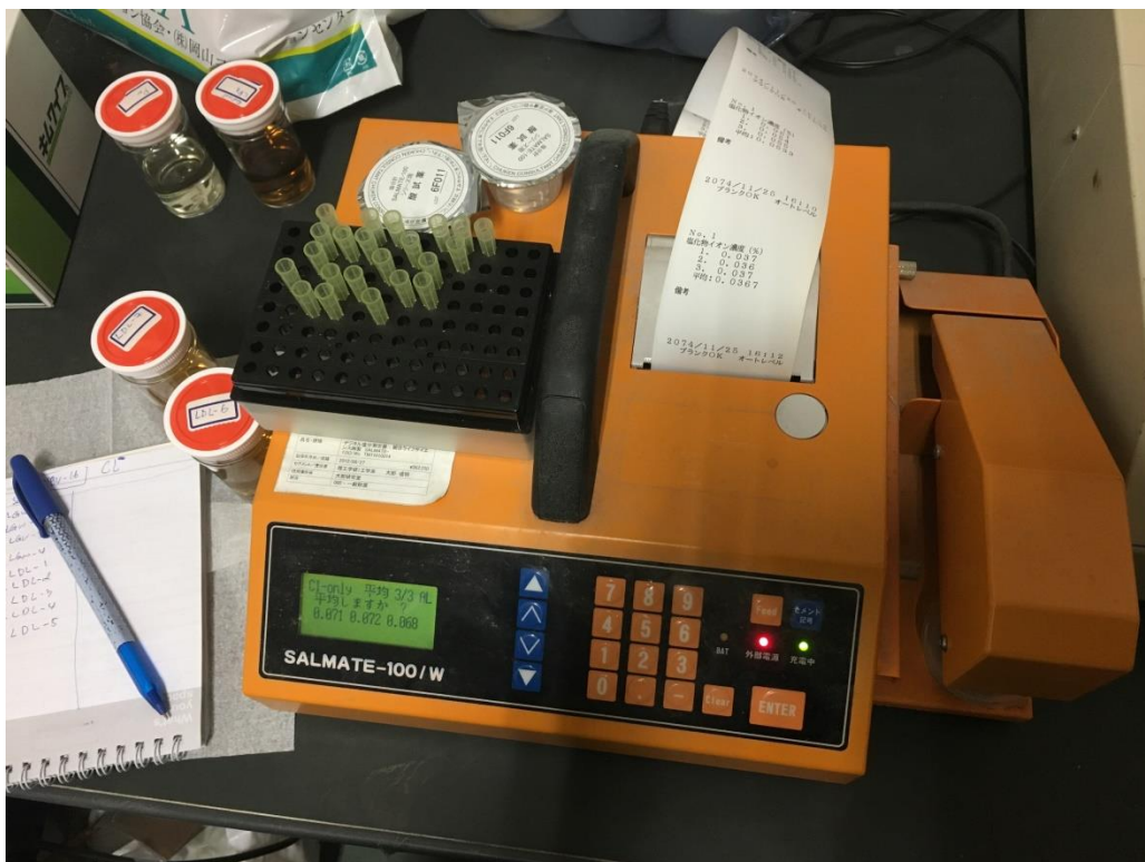
Figure 4.5 SALMATE-100/W for Cl measurement
