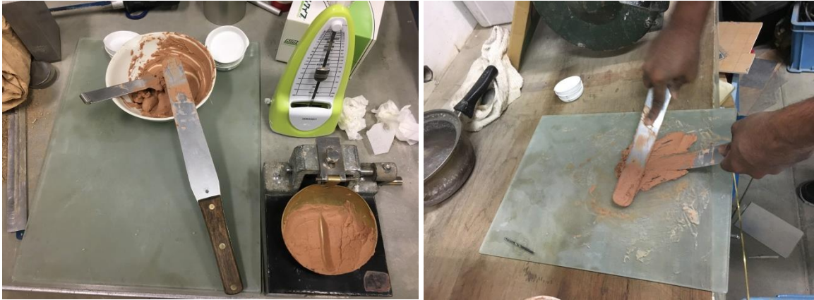
Figure 3.18 Atterberg limit (LL and PL)
