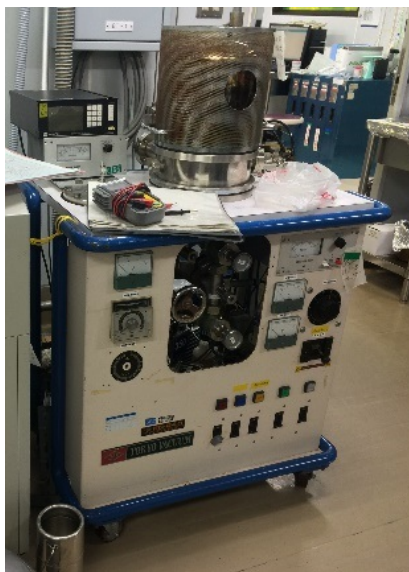
Figure 4.10 Thermal evaporation system (TOKYO VACUUM, EG-240).
