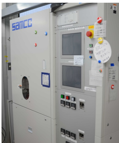
Figure 4.11 Plasma-enhanced chemical vapor phase deposition (PECVD) system (SAMCO;PD-240).
