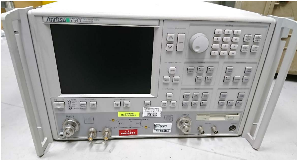
Figure 4.51 Vector Network Analyzer(Anritsu 37397C,40 MHz-65 GHz).
