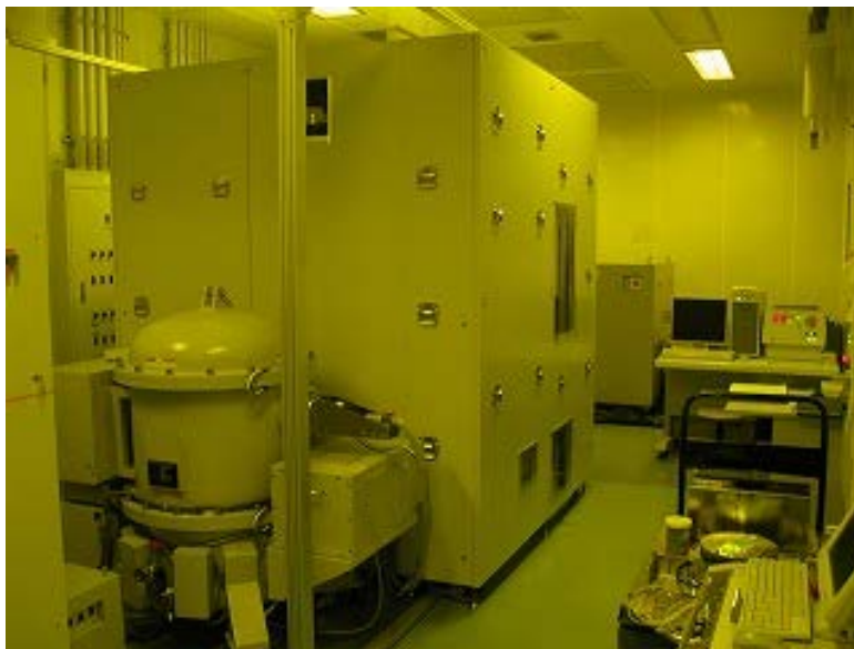
Figure 4.8 Appearance of electron-beam lithography system of JEOL JBX-6300FS.
