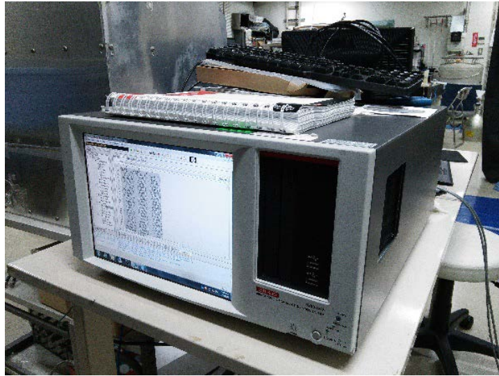
Figure 5.12 Semiconductor parameter analyzer (Keithley, 4200-SCS)
