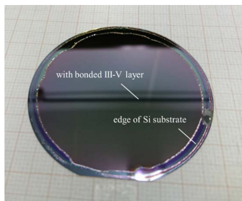
Figure 4.15 Fabricated 2-inch membrane III-V layer on a Si substrate by BCB bonding.
