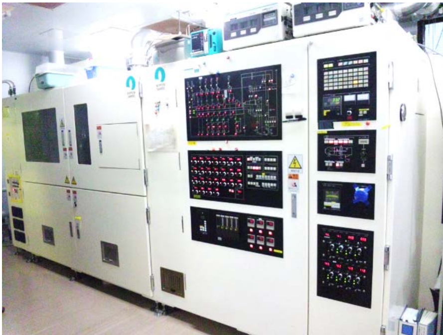
Figure 3.23 OMVPE equipment of HR3255.
