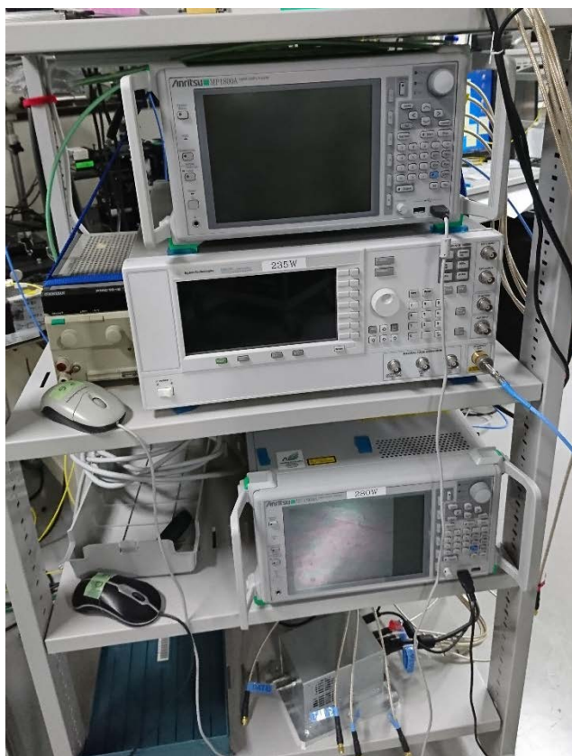
Figure 4.61 MP1800A Signal Quality Analyzers implementing MU181020B, MU182021A, MU181040B, and MU182041A.
