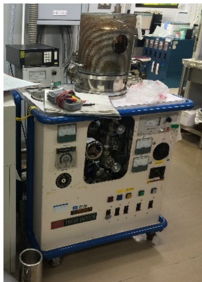
Figure 4.10 Thermal evaporation system (TOKYO VACUUM, EG-240).
