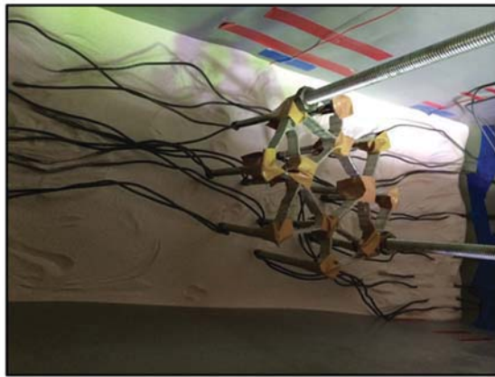
(b) Piles fixed at box center during sand pouring.
