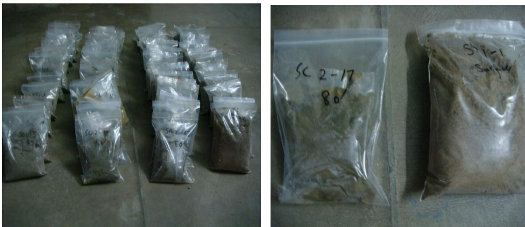
Fig. 4.24: Soil collection and sampling during soil boring (Picture taken in June 2009)
