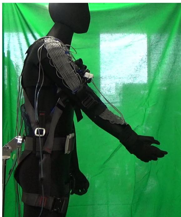
Fig. 1: Side view of the soft power support suit for upper limbs
