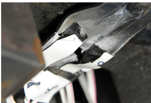
(g) Girder initial crack on the left end (1/33rad-29cycle)
