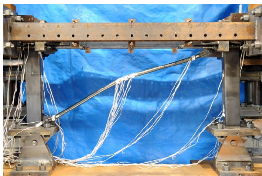
(a) Brace global buckling (1/100rad-1cycle)
