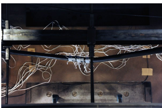
(e) Deformation condition of the global buckling (150 % - 2nd)
