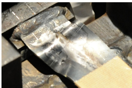
(g) Girder local buckling (after testing, left end)
