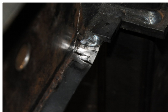
(h) Girder cracking point on the left end after testing
