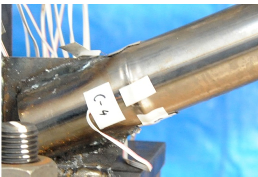
(c) Brace local buckling on the end part (1/50rad-2cycle)
