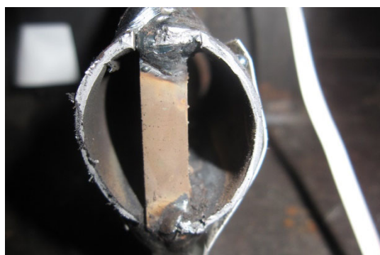
(c) Fracture section of brace end (After testing)
