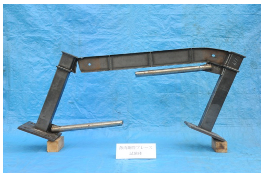
(e) Collapsed specimen after testing
