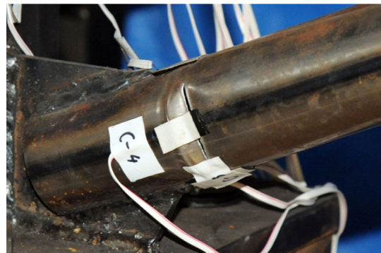
(f) Brace initial crack on the end part (1/33rad-8cycle)
