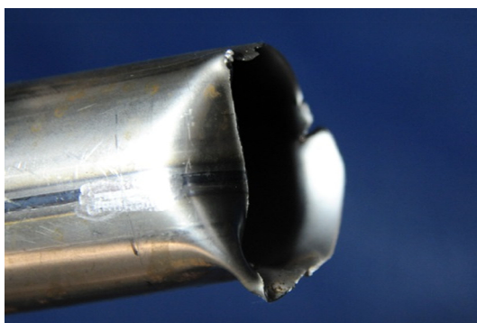
(g) Fracture section (after testing, left side)
