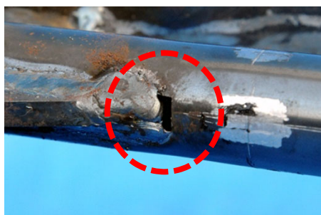
(a) the specimen including partial loss of section area
