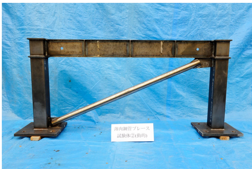
Photo 2.3.1 Specimen before shake table testing
