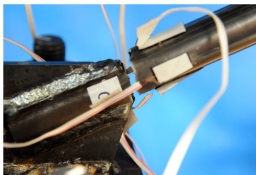
(b) Gross section fracture of brace end (1/33rad-1cycle)
