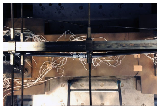
(b) Deformation condition of the global buckling (100 % - 2nd)
