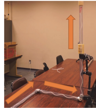
(c) Locomotion in a practical piping system
