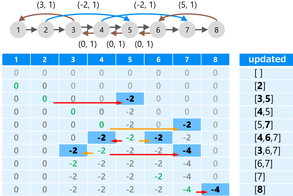
Figure 5.5: An example of execution with a priority queue (“updated”). The (cost, capacity) labels are shown for valid edges. Edges without labels have (0, \infty) . The cell at row i and column j of the table shows the cost(j) at step i . The cells updated in each step are highlighted.
