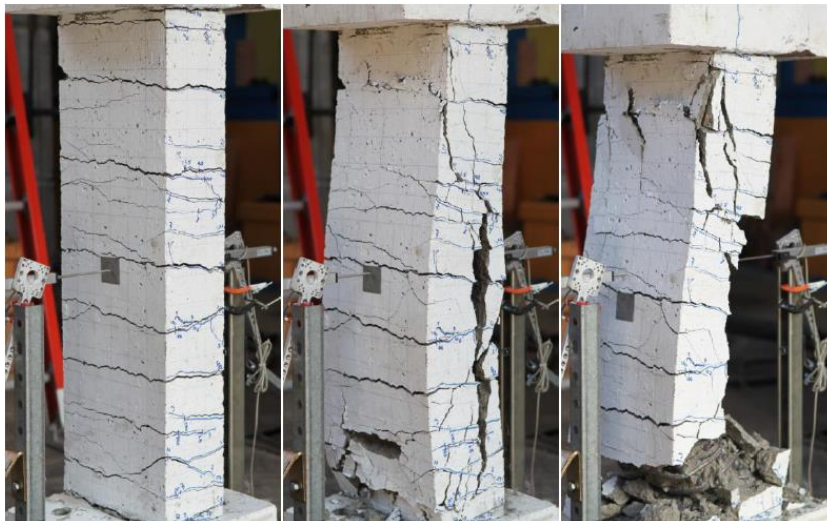
Figure 2.13 - Failure progression of Specimen S1 (Compression Loading after 4% Tensile Excursion) (Creagh et al. , 2010)
