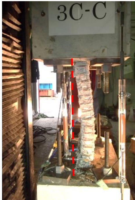
Figure 4.1 –Final buckling shape of 3C-C
