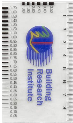
(a) Crack gauge card
