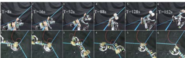
Fig. 12 Dual Arm Type on Spatial Tilting
