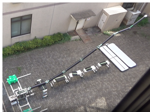
Fig. 3 Experiment on keeping horizontal posture
