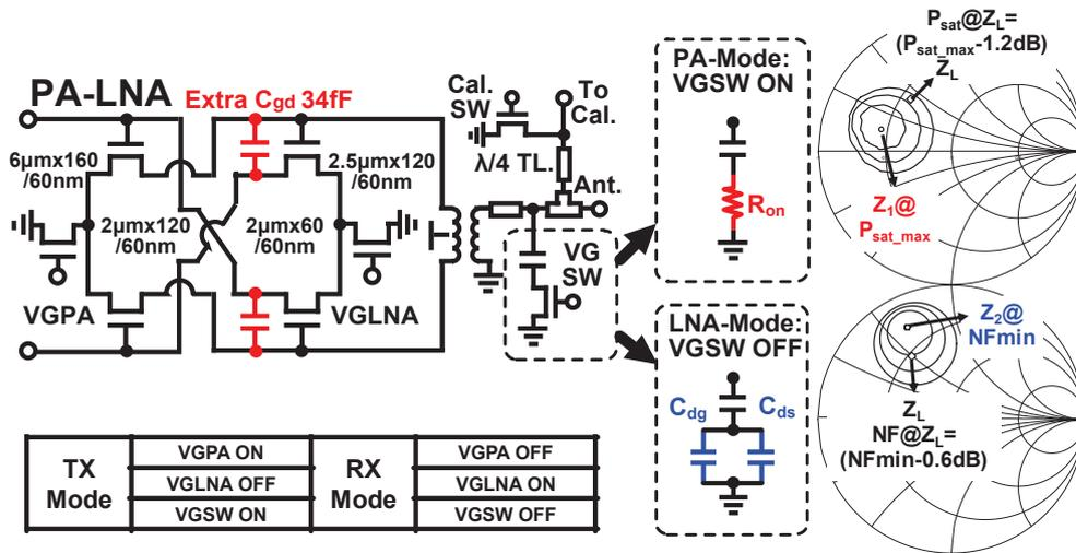
Figure 6.7: Circuit schematic of the proposed PA-LNA.
