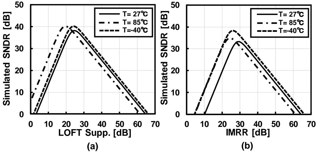
Figure 3.8: Simulated SNDR of the calibration path against (a) LOFT suppression and (b) IMRR.
