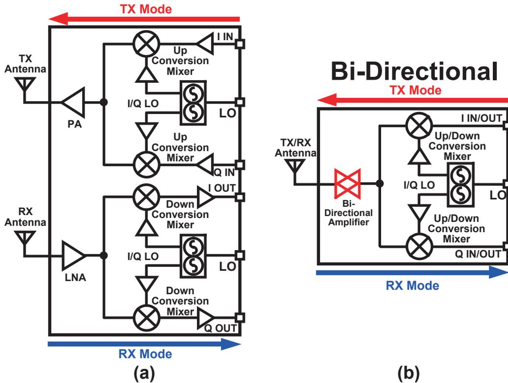
Figure 4.1: Block diagrams of (a) conventional 60-GHz direction-conversion transceiver and (b) bi-directional transceiver.
