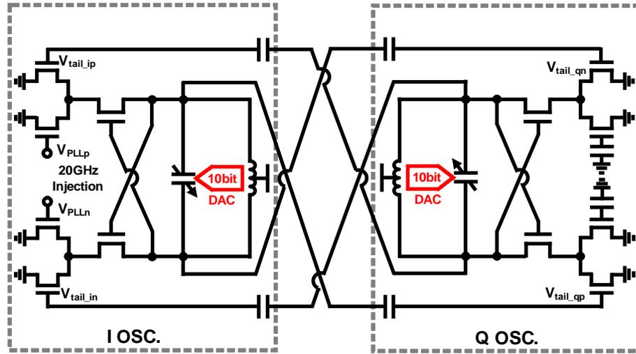
Figure 3.10: Circuit schematic of quadrature injection-locked oscillators (QILO).
