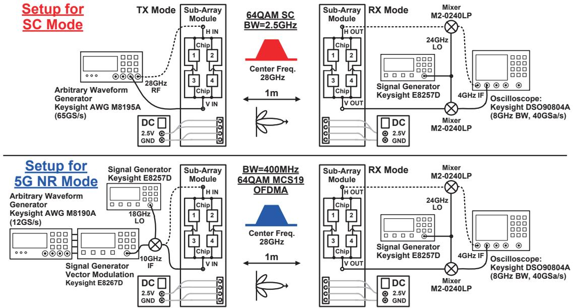
Figure 6.18: Measurement setup for the OTA measurement.
