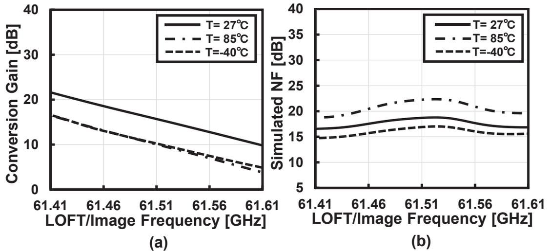
Figure 3.7: Simulated (a) conversion gain and (b) noise figure of the proposed calibration block against the input impairment frequency of the TX.
