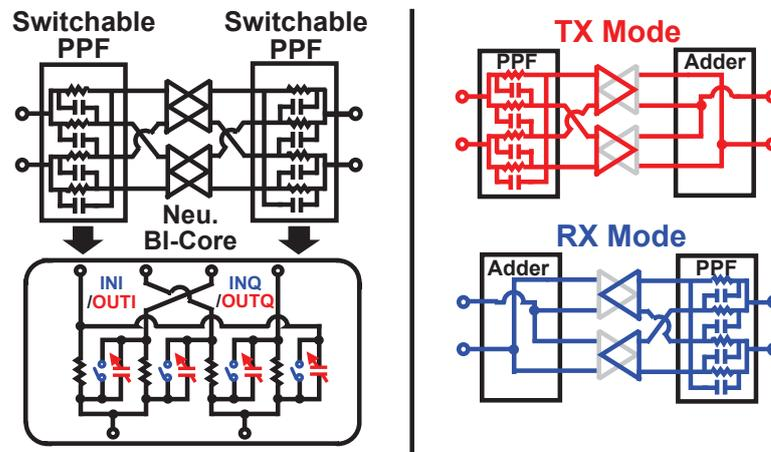
Figure 6.10: Circuit schematic of the proposed active bi-directional phase shifter.
