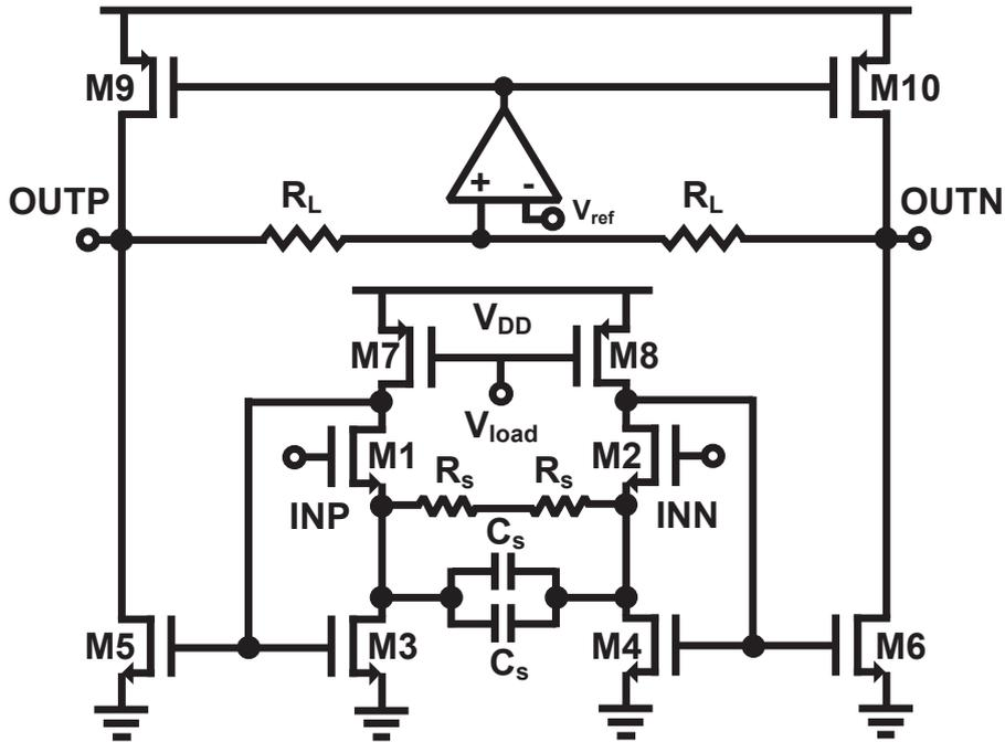
Figure 3.15: Circuit schematic of the baseband amplifier.
