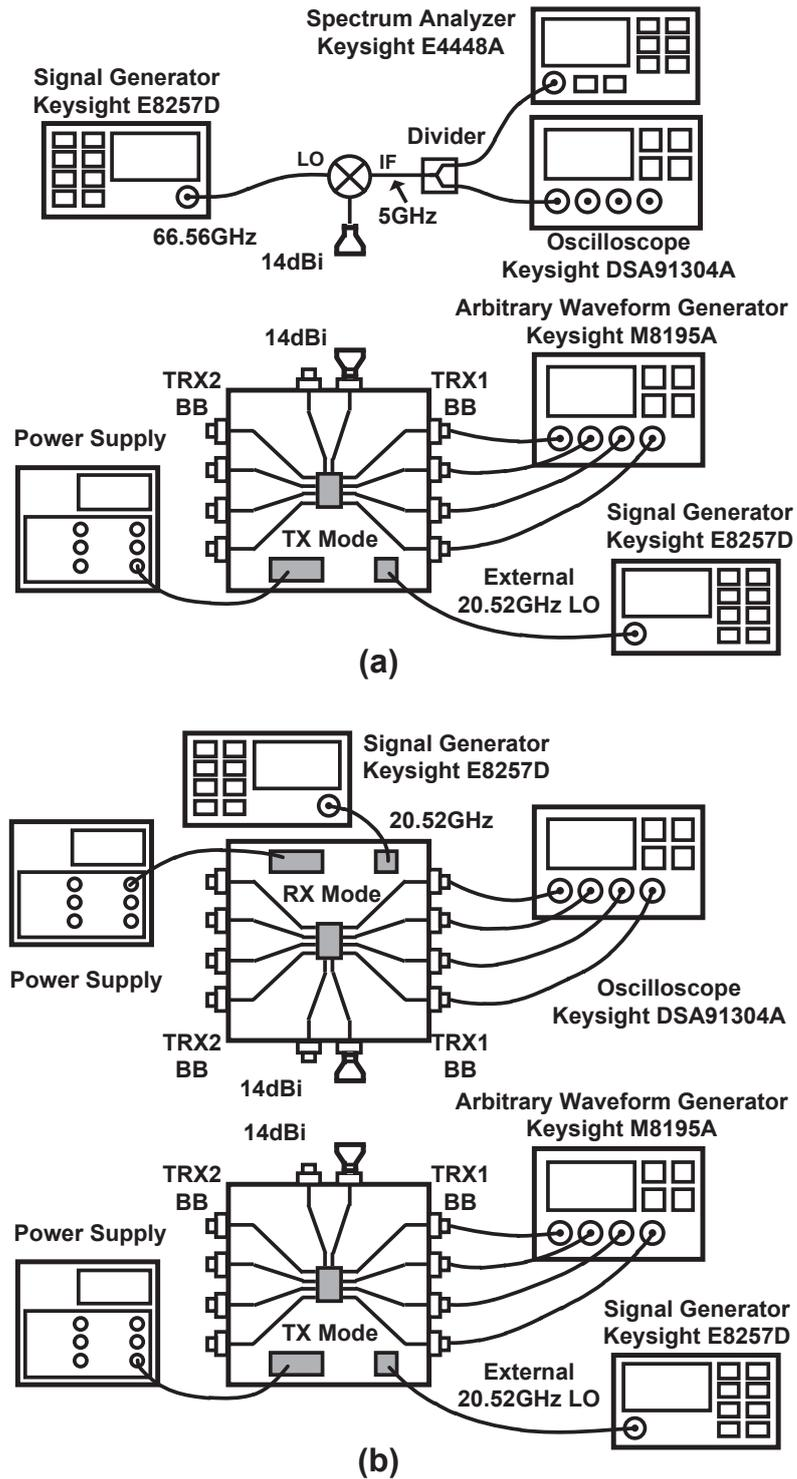
Figure 4.20: Equipment setups for (a) TX spectrum, constellation, and EVM measurement and (b) TX-to-RX constellation and EVM measurement.
