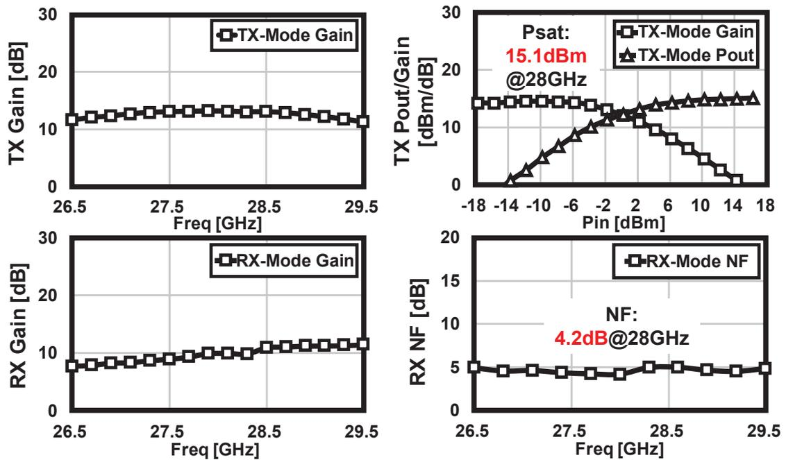
Figure 6.13: Measured on-wafer characteristics of the single-path beamformer.
