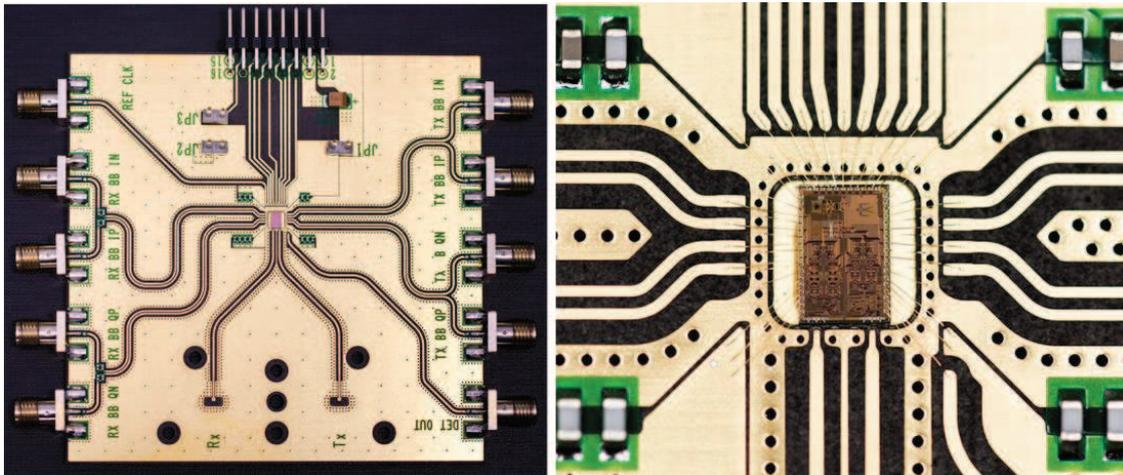
Figure 3.20: RF PCB for measurement.
