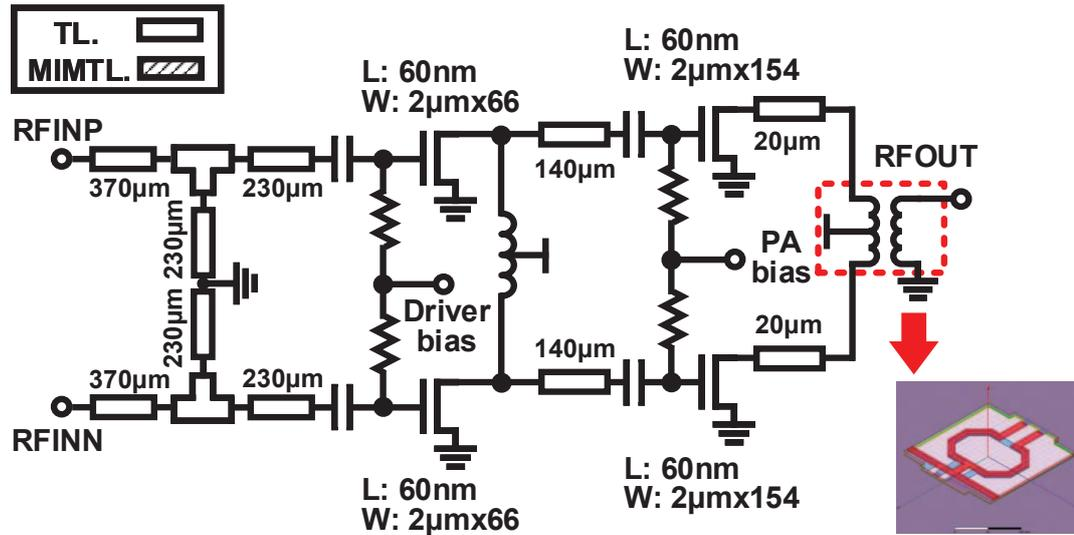
Figure 5.13: Circuit schematic of differential power amplifier.
