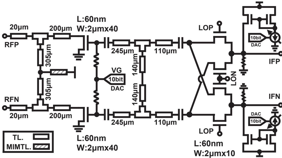
Figure 5.12: Circuit schematic of up-conversion mixer and RF VGA.
