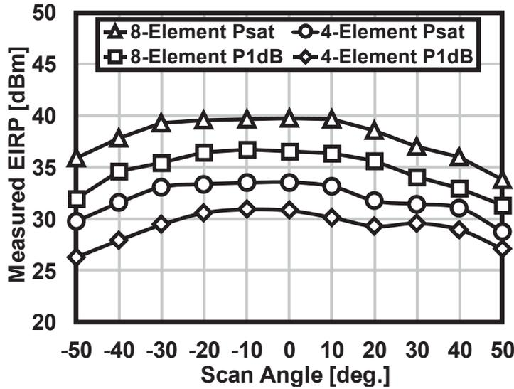
Figure 5.23: Measured EIRPs for (a) four-element and (b) eight-element phased-array transceiver modules.
