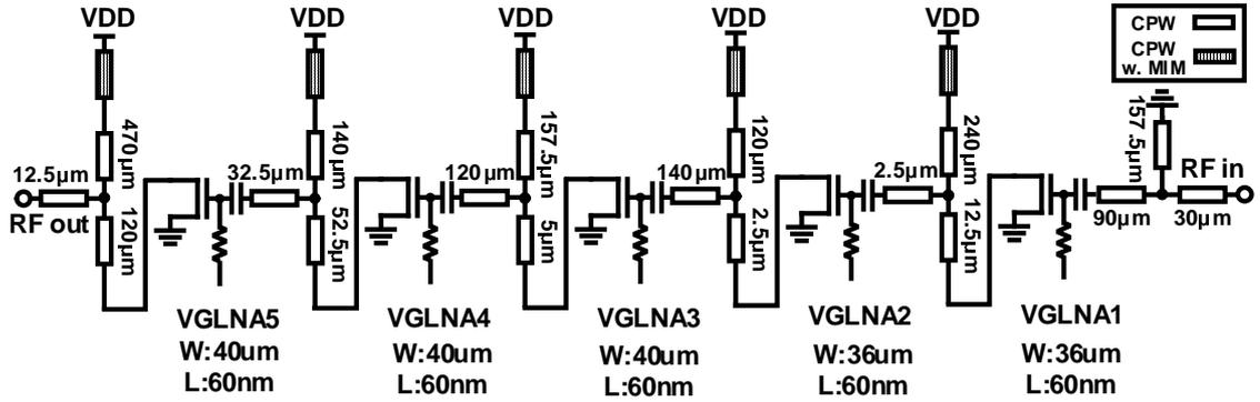
Figure 3.18: Circuit schematic of the 60-GHz 5-stage LNA.
