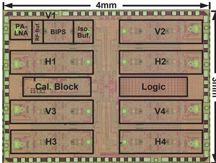
Figure 6.12: Die micrograph of the proposed chip.
