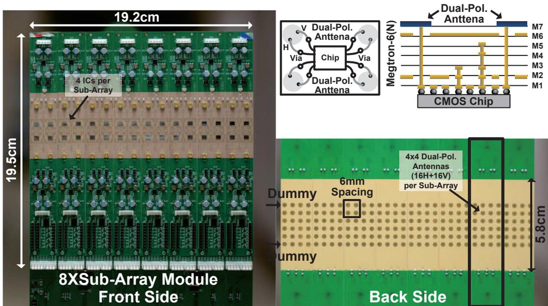
Figure 6.16: Photograph of the transceiver module.
