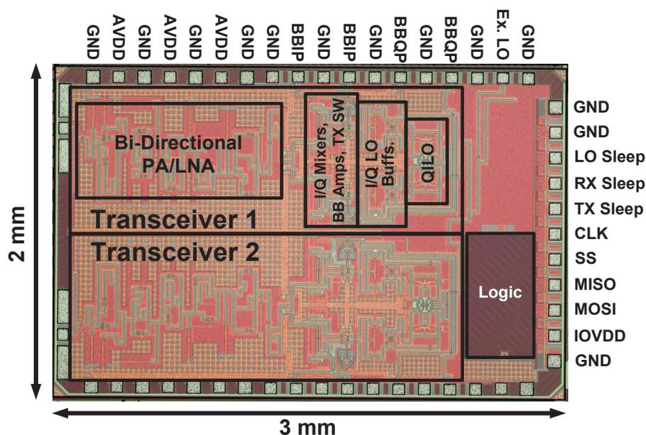
Figure 4.16: Die micrograph of proposed bi-directional transceiver chip.
