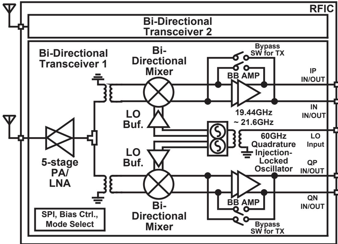
Figure 4.3: Block diagram of proposed bi-directional transceiver.
