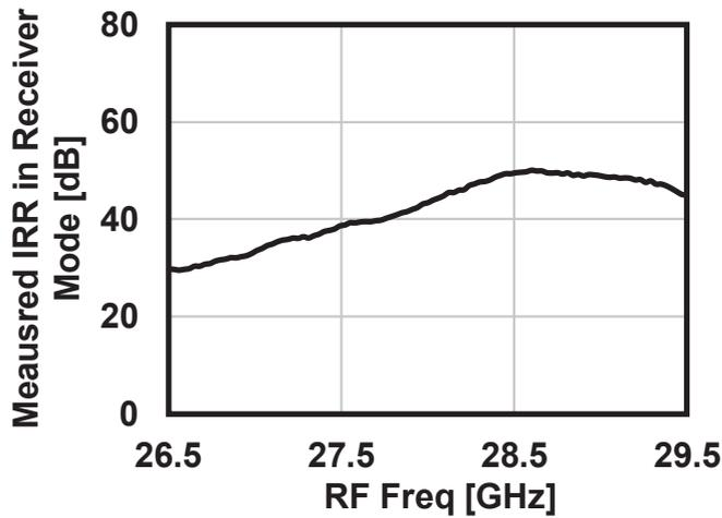
Figure 5.16: Measured receiver-mode IRR against input RF frequency.
