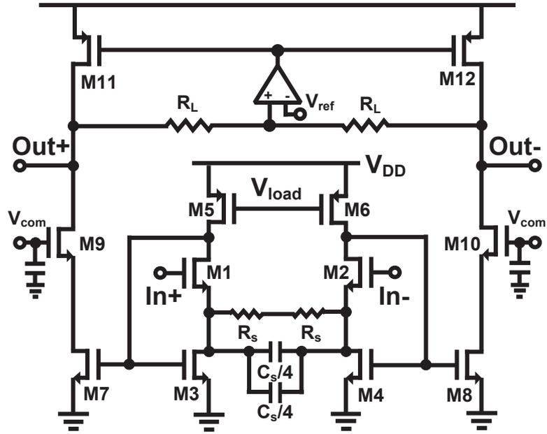
Figure 4.11: Circuit schematic for first stage of baseband amplifier.
