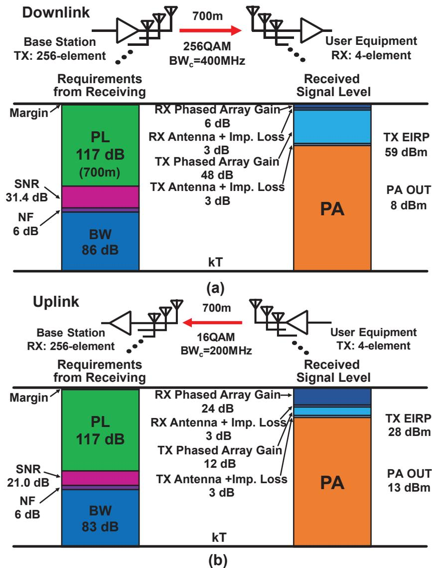
Figure 2.8: Link budget examples for (a) 5G downlink and (b) 5G uplink.
