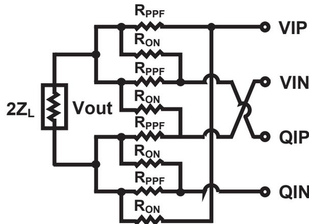
Figure 7.2: Circuit schematic for the adder-mode switchable PPF.
