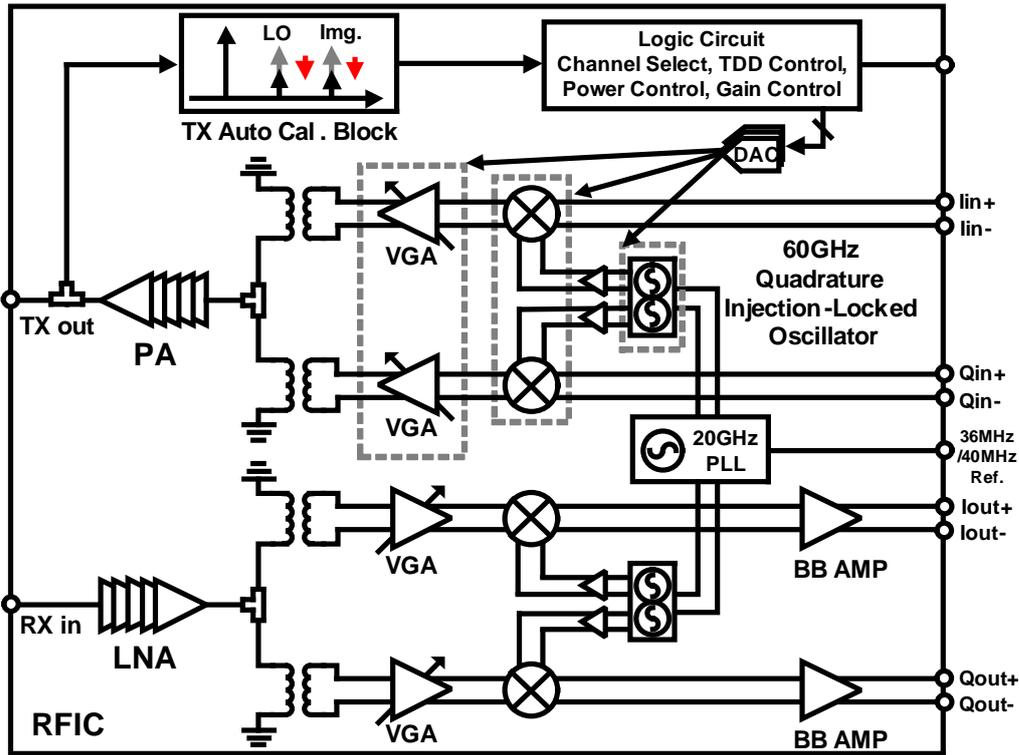
Figure 3.3: Block diagram of the proposed 60-GHz transceiver.
