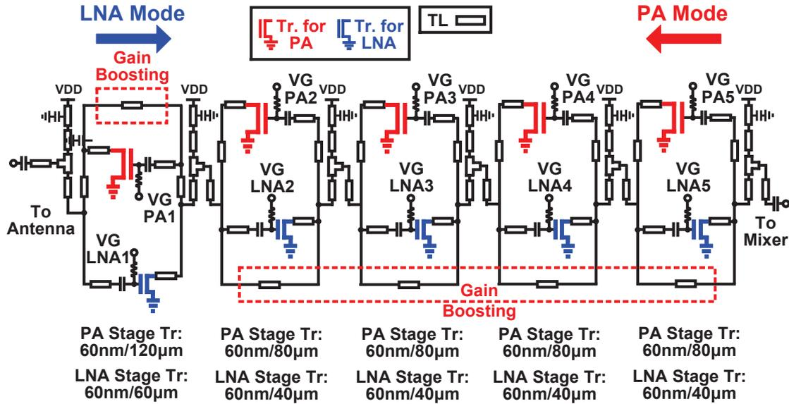
Figure 4.7: Circuit schematic of proposed five-stage PA-LNA.
