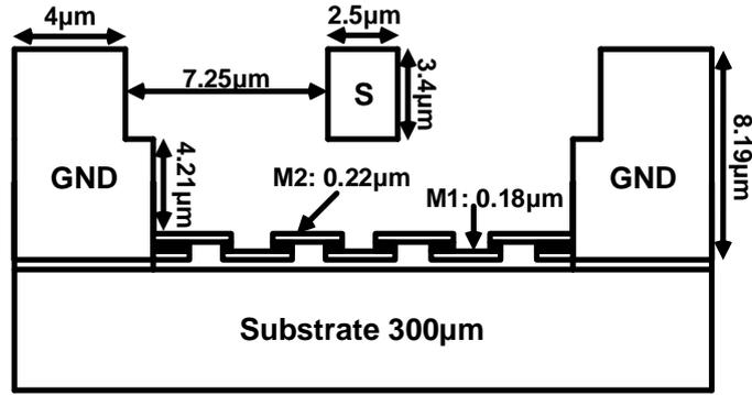
Figure 3.13: Cross-section view of the transmission line.
