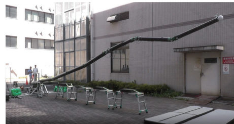
Fig. 19. Experiment on keeping the horizontally extended posture using the 10 m model.
