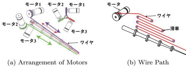
Fig.3. Bending Mechanism
