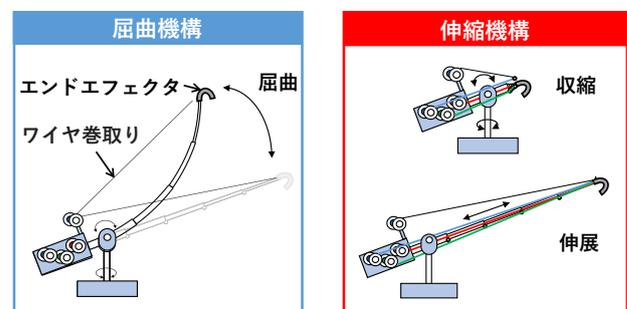
Fig.1. Mechanism of Elastic Telescopic Arm
