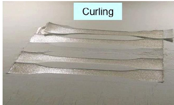
Fig. 8: Problems observed during SLS processing: “curling” [19]
