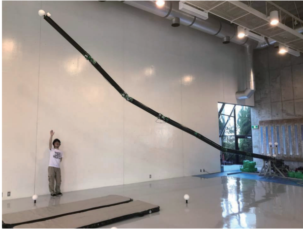
Fig. 16 Experiment on keeping the horizontally extended posture using the 10 m model.
