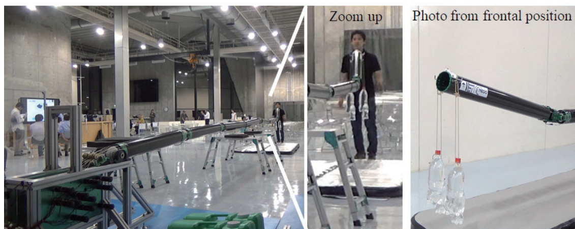
Fig. 22 Payload testing experiment. The bottled water of 4.4kg were attached at the tip of the arm.
