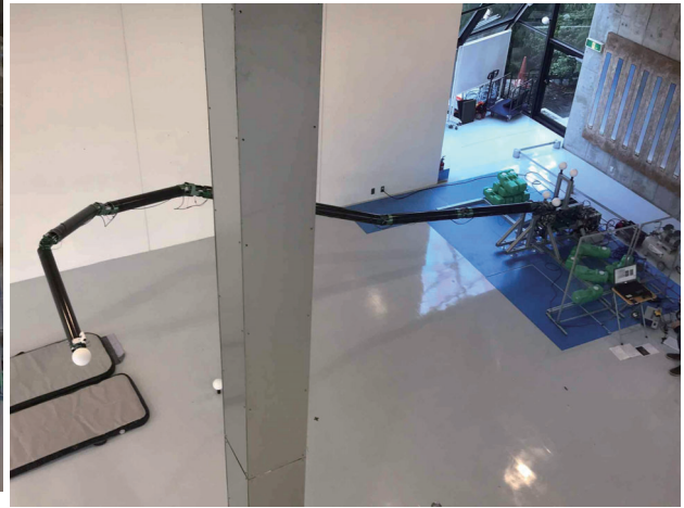
Fig. 17 Experiment on keeping the yaw bending posture using the 10 m model.
