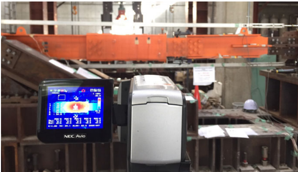
Figure 3. Thermal imaging device capturing the damper temperature during long-duration loading test.
