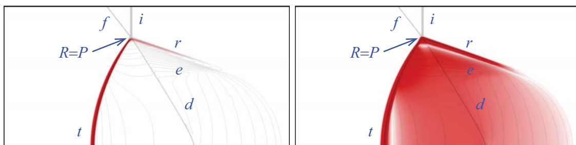
Fig.3.6: Shock-interface interaction structure with \alpha = 38 deg. Legends are same as Fig. 3.5.
