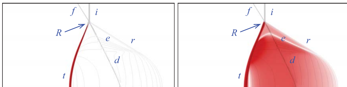
Fig.3.5: Shock-interface interaction structure with \alpha = 32 deg. Interval of contour lines is 0.01 \text{ kg/m}^3 . And maximum and minimum values of white-red colormap are 300Pa and 2000Pa (left), 0Pa and 200Pa (right) respectively.
