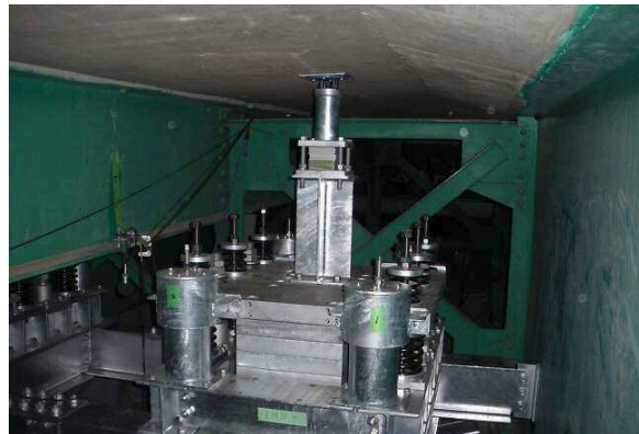
(b) Impact Mass Damper (IMD)
