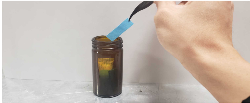
Step 1 Take out the humidity test paper [手順① 乾燥度試験紙を取り出す]
