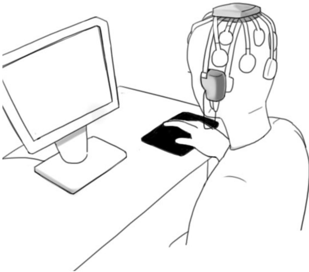
Figure 2.1: Experimental environment. Subjects sat in a comfortable chair in front of a monitor on a desk with a touch pad. They adjusted their seat and the position of the touch pad to their comfort. Subjects wore a Quick-30 Dry EEG Headset (Cognionics, Inc.) to measure EEG signals. Subjects operated the touch pad with their finger.
