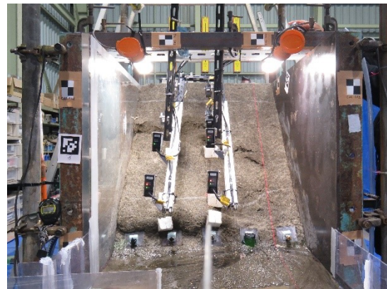
(d) Deepening of the cracks on upper surface with limited soil mass movement (800 mm water level)
