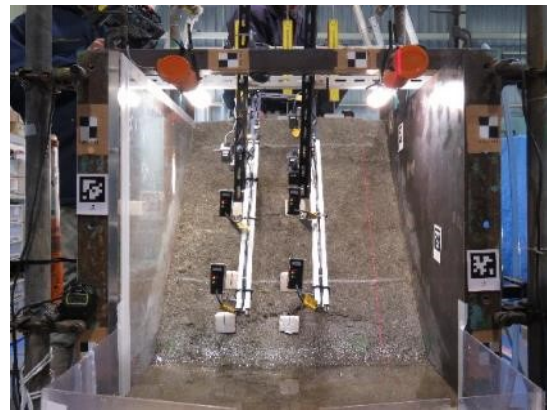
(b) Appearance of the crack near the toe region (at 700 mm water level)
