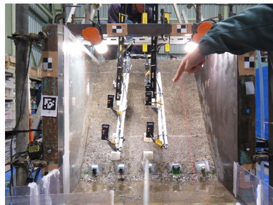
(b) Appearance of small cracks above near toe (700 mm to 800 mm water level)
