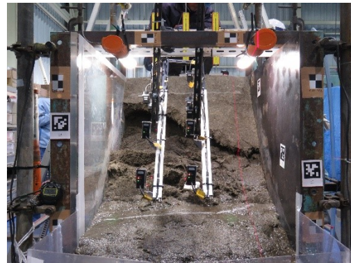
(d) Soil mass movement with deep sliding surface ((800mm-900 mm water level)
