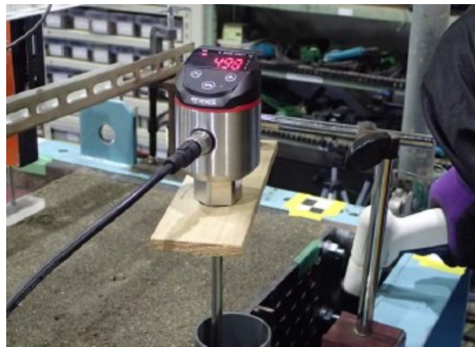
Figure 3.3 Water level meter (FL-001) used for measuring flood water level.
