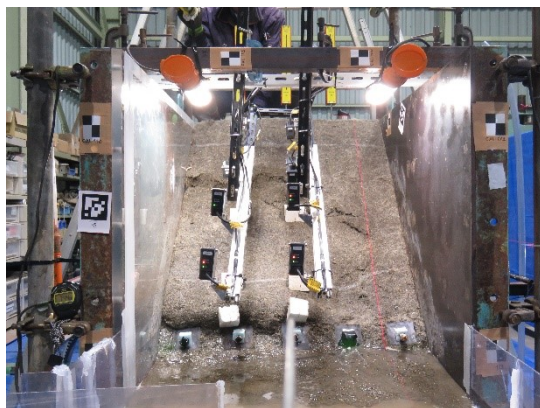
(c) Formation of arch above the pipe location (800 mm water level)
