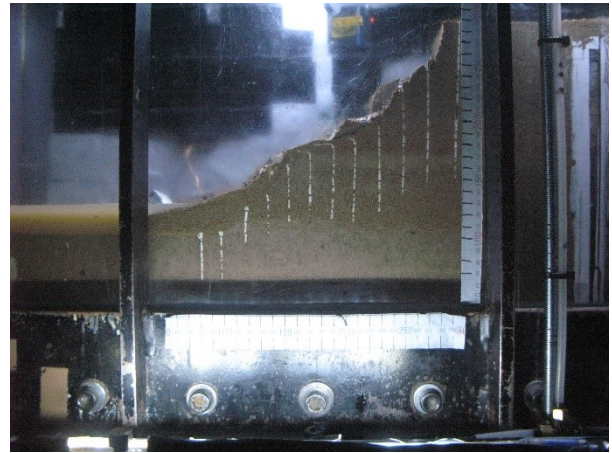
Formation of cracks on crest showing large deformation
