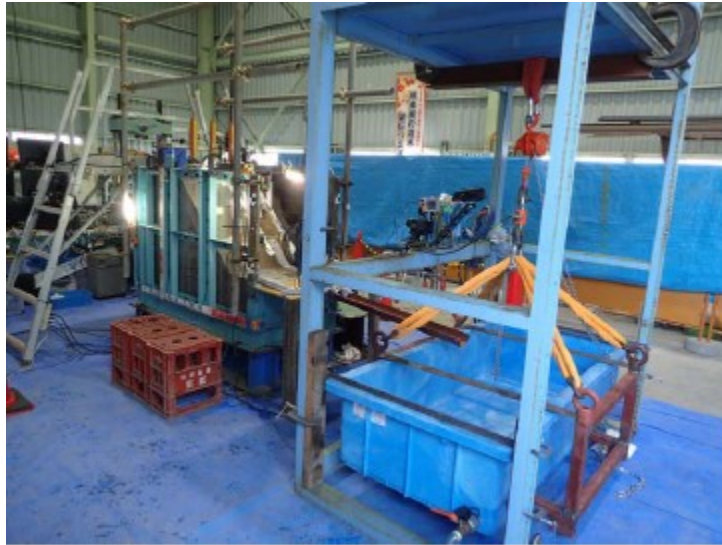
Figure 3.4 Arrangement for collecting and measuring the drained seepage water
