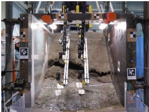
(c) Progression of failure to upper region of the slope (800mm-900 mm water level)
