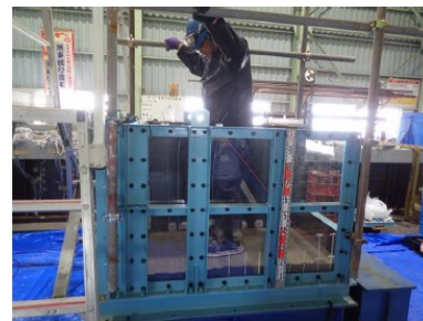
(b) Manual compaction of the soil layer
