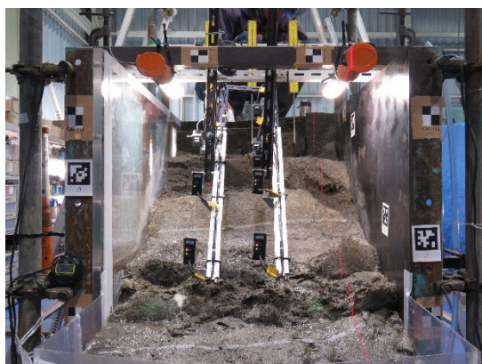
(e) Complete collapse of the soil slope (900 mm water level)
