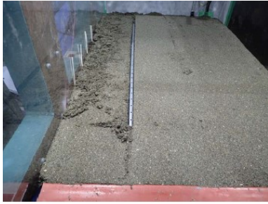
(e) Placement of pipe
