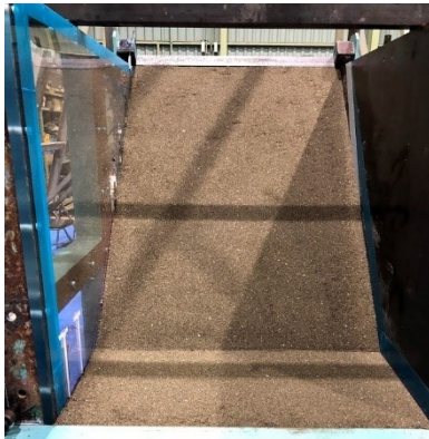
(g) Soil Slope after excavation
