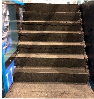
(f) Completion of compaction of soil layers
