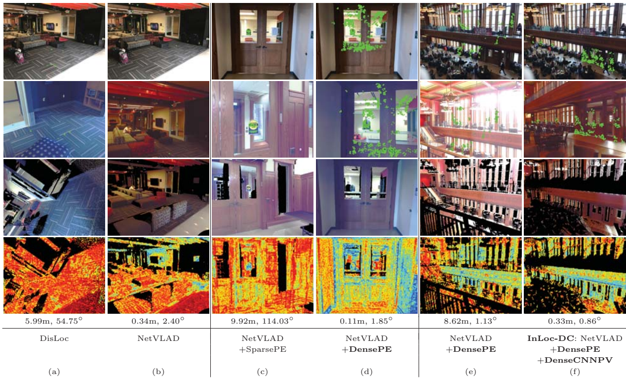
Figure 4.10: Qualitative comparison of different localization methods (columns). From top to bottom: query image, the best matching database image, synthesized view at the estimated pose (without inter/extra-polation), error map between the query image and the synthesized view, localization error (meters, degrees). Warm colors on the error map correspond to large errors. Green dots are the inlier matches obtained by P3P-LO-RANSAC.
