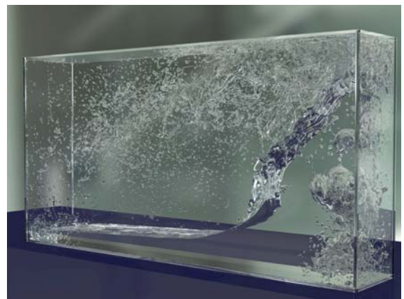
Fig.2.66: The predicted time evolution of gas-liquid in the case of L = 0.018 \text{ m} , obtained at 1152 \times 192 \times 576 meshes for the dam breaking onto wet floor problem.
