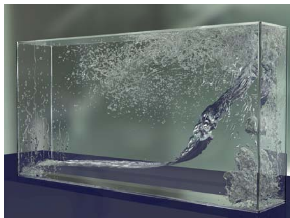
Fig.2.66: The predicted time evolution of gas-liquid in the case of L = 0.018 \text{ m} , obtained at 1152 \times 192 \times 576 meshes for the dam breaking onto wet floor problem.
