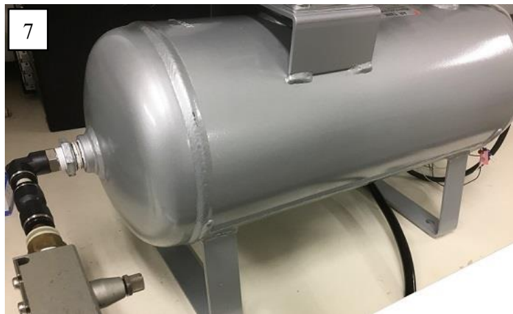
Fig.2-6 An air tank with 10 dm 3 volume
