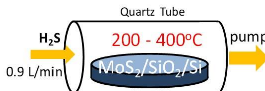
Figure 3.3 Schematic illustration of H 2 S annealing [3.4].
