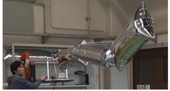
Figure 17. Complete three-link arm.
