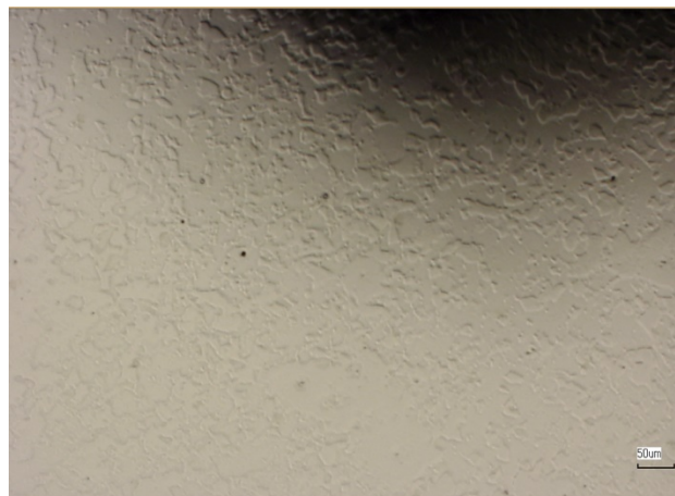
Fig.2. 22 Optical image of surface morphology of the plated Ni-P layer
