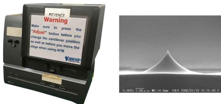
Fig.2. 9 the AFM device and the morphology of the tip of the probe
