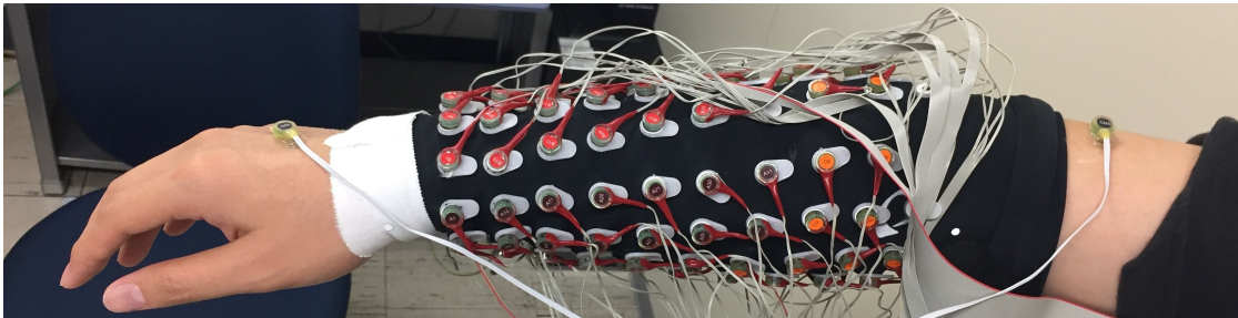
Figure 4.17: Example of bio-semi electrode sensor in first experiment, other experiment also use the same pattern, please notice the CMS and DRL electrodes. The location of this electrodes need to changes according to subject with 1. on the back of hand 4 centimeters apart, 2. between the hand and upper arm, 3. in position A26 and B26.
