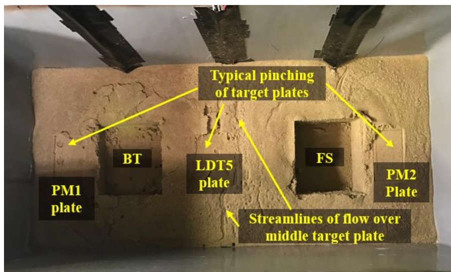
Fig. 5.14. Model ground surface after the experiment. Pinching of target plates and trace of water flow is visible.
