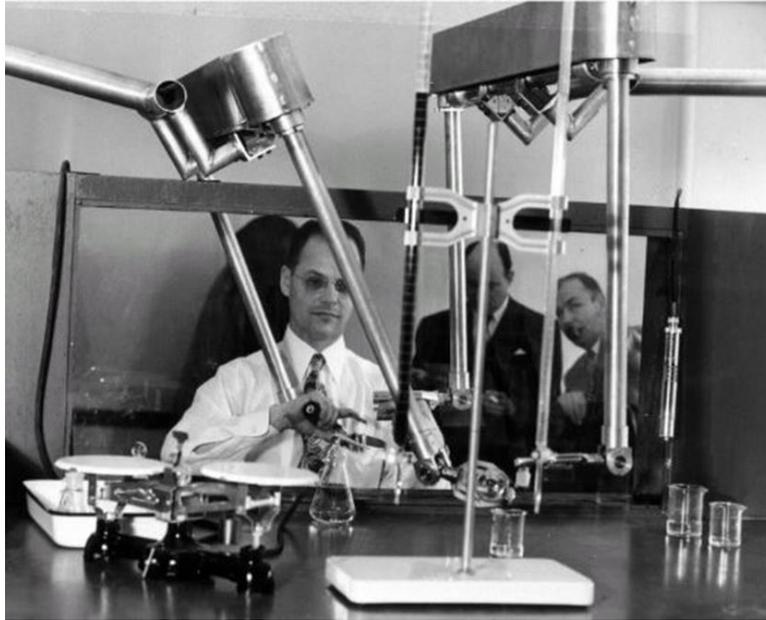
Fig. 1.1 The first master-slave manipulator “model M1” [1].
