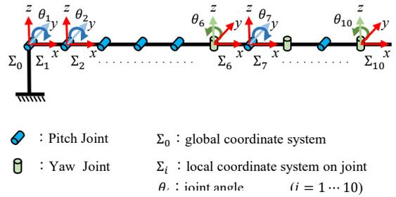
Fig. 2 Joint configuration.
