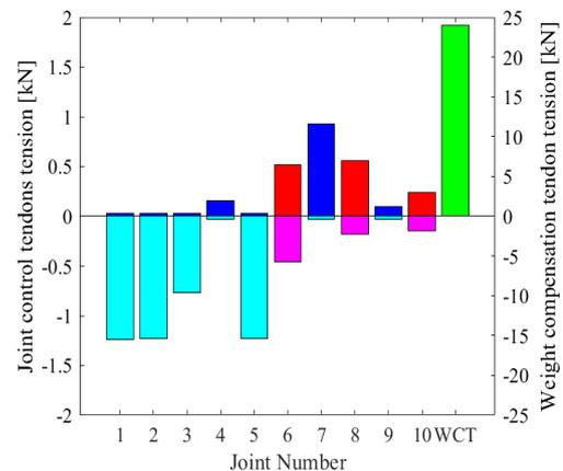
Fig. 11 Tension of tendons when WCT is 25 kN.
