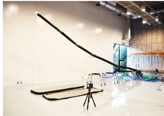
Fig. 1 Super Dragon: a 10 m-long coupled tendon-driven manipulator.
