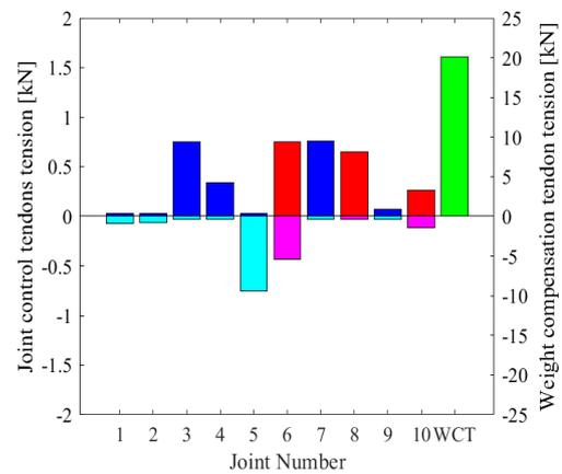
Fig. 10 Tension of tendons when WCT is 20 kN.
