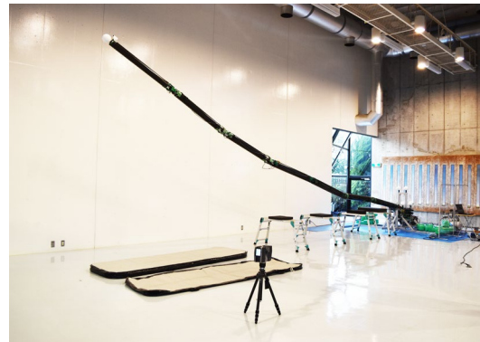
Fig. 1 Super Dragon: a 10 m-long coupled tendon-driven manipulator.
