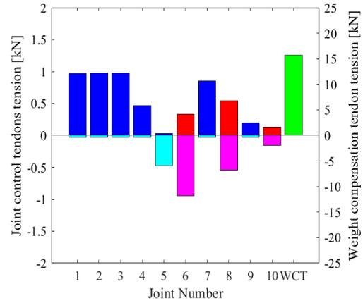
Fig. 9 Tension of tendons when WCT is 15 kN.
