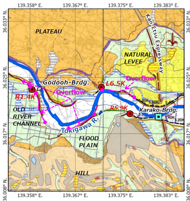
Fig. 9. Landform classification map for flood control in vicinity of breaches. The landform classification map was obtained from the base map information of the Geospatial Information Authority of Japan ( https://cyberjapandata.gsi.go.jp/xyz/lcmfc2/13/7267/3216.png ).
