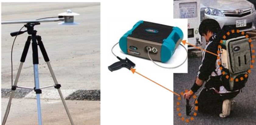
Figure 3 Albedo and reflectance observed directly in situ using pyranometers (left) and spectroradiometers (right), respectively.
