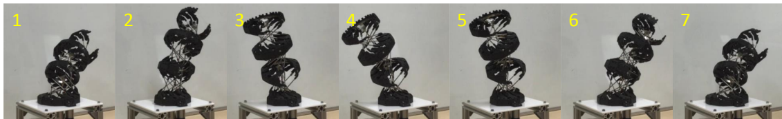
Figure 4.18: Swinging from right to left and vice versa. When l_{\text{wire},0L} is longer than l_{\text{wire},0R} , the prototype tilts to the right. Conversely, when l_{\text{wire},0R} is longer than l_{\text{wire},0L} , the prototype tilts to the left.
