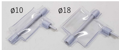
Figure 5.12: Two types of airbags made by PVC
