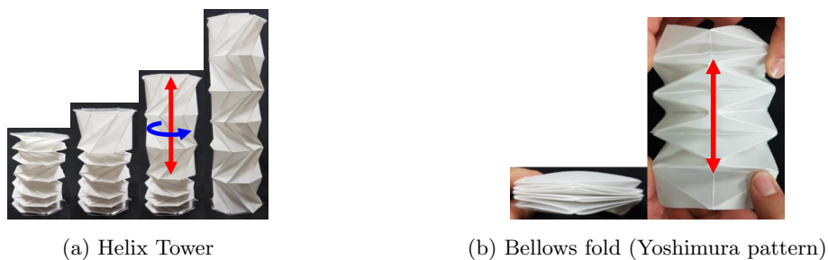
Figure 1.1: Representative deployable cylindrical origami structures. These structures can be extended by pulling them along the longitudinal direction and/or rotating each segment.
