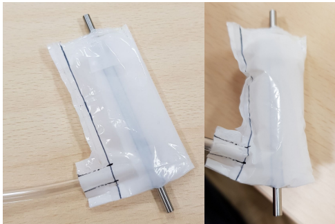
Figure 5.18: Airbag made by polyethylene sheet
