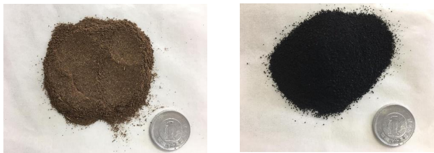
Figure 2.2 Palm kernel shell (left) and chemically treated palm kernel shell (right) prior to pyrolysis
