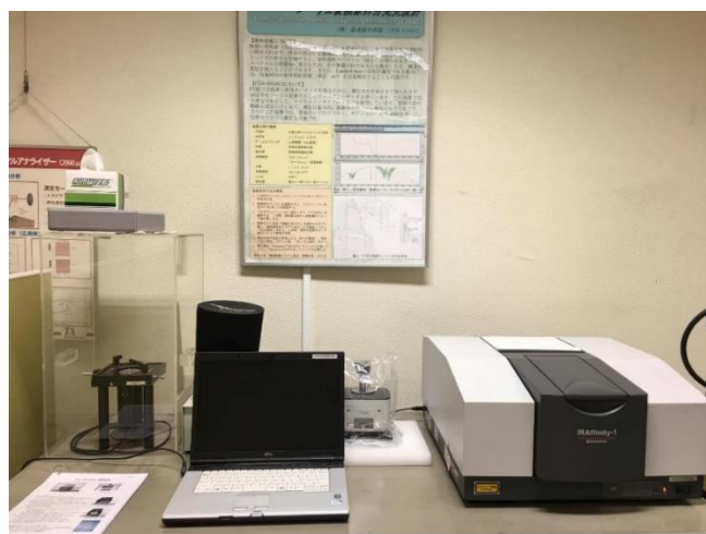
Figure 3.4 Infrared spectrometer IRAffinity-1 (Shimadzu, Japan) for surface functional groups analysis of PKSAC
