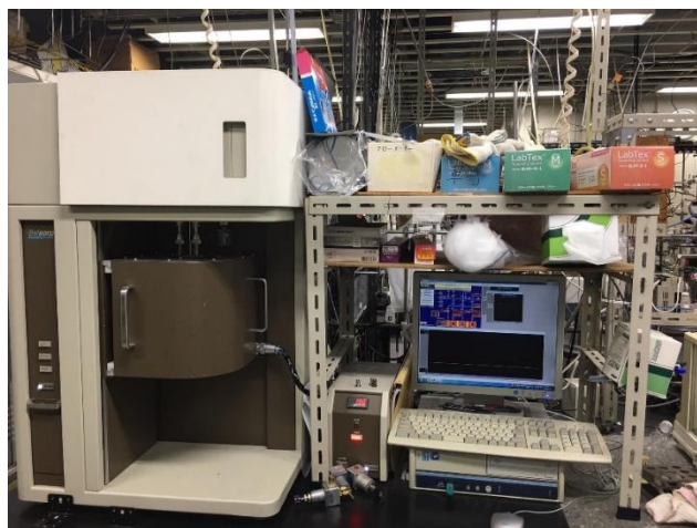
Figure 3.3 BELSORP-max: BEL JAPAN for specific surface area and porosity properties analysis of PKSAC
