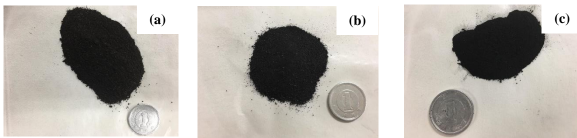
Figure 3.9 Appearance of PKSAC produced from different H_3PO_4 concentrations (a) c_P= 2 \text{ kmol m}^{-3} (b) c_P= 4 \text{ kmol m}^{-3} (c) c_P= 8 \text{ kmol m}^{-3} )
