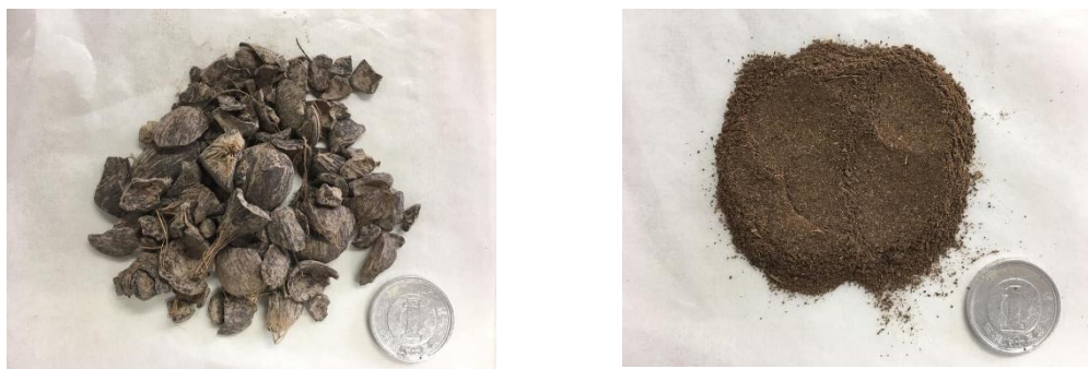
Figure 2.1 Appearance of palm kernel shell (left: raw palm kernel shell right: sieved palm kernel shell)
